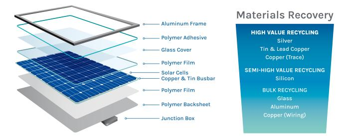
**Figure 5. S**chematic of solar panel materials and which materials are captured in different types of recycling processes. The materials are divided into categories according to their value after recycling.
